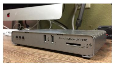
A Canon FX1 camera is connected to an iMac® running ProPresenter media presentation software, which mixes the video feed with its lower thirds (lyrics, verses) along with audio from the sound board (x32), then sends it out as an HDMI feed that goes into the Monarch HDX. MediaFusion provides Lifehouse Church with the necessary content delivery services.
