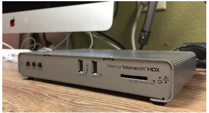
A Canon FX1 camera is connected to an iMac® running ProPresenter media presentation software, which mixes the video feed with its lower thirds (lyrics, verses) along with audio from the sound board (x32), then sends it out as an HDMI feed that goes into the Monarch HDX. MediaFusion provides Lifehouse Church with the necessary content delivery services.
